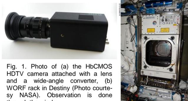
Fig. 1. Photo of (a) the HbCMOS HDTV camera attached with a lens and a wide-angle converter, (b) WORF rack in Destiny (Photo courtesy NASA). Observation is done through the window.
